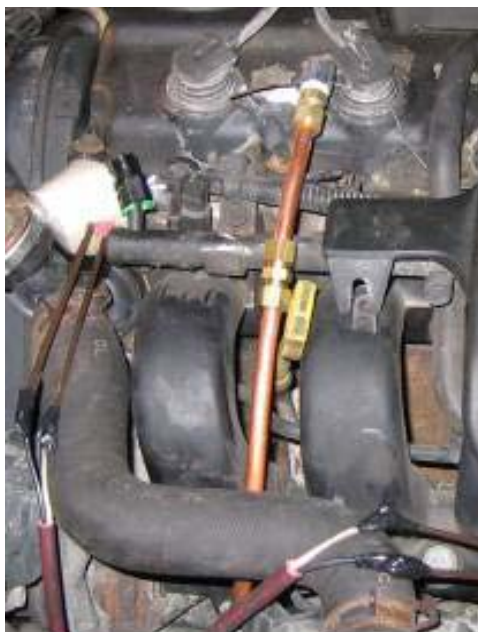
Figure 4-15: Automobile engine compartment fire initiation device.
