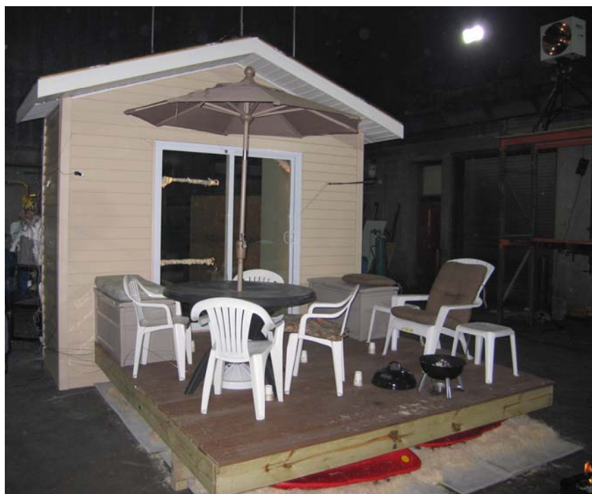
Figure 4-10: Photograph showing the composite deck scenario with furnishings.
