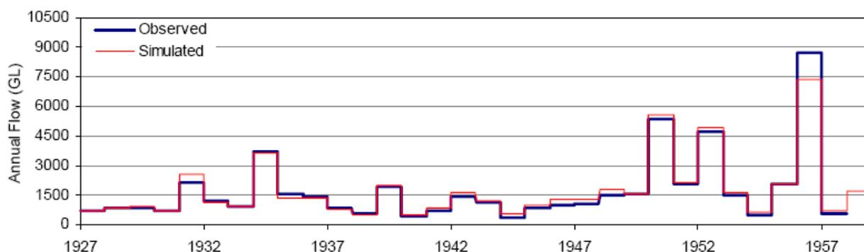
Figure 1 Calibration results for the Upper Murrumbidgee model (CSIRO, 2008)
