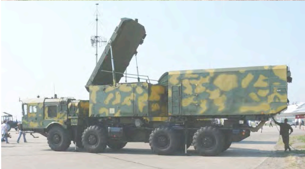
5P85TE2 towed and 5P90S self-propelled launchers, and 92N6 GRAVE STONE engagement radar components of S-400 batteries.
