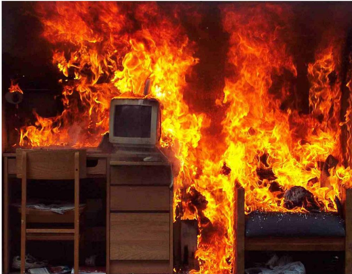
Figure 14 The fire spread is rapid and dramatic. Within approximately five minutes the room's contents are fully involved.
