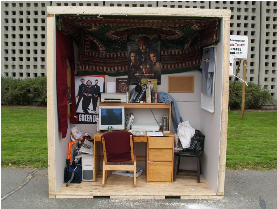
Figure 11 One of the important considerations when doing a burn is to have plenty of fuel and a continuous fuel path up to the ceiling tapestry. It is also important to make sure that the room is not packed too full with furniture and that there isn't enough airflow. In this mockup, the fire is going to start in a trash can in the lower left corner and travel up the posters and wall hanging to the tapestry.
