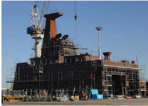
Figure B - Aft superstructure block under construction in Spain. Australian construction of this block required it to be constructed and lifted as four separate blocks due to manufacturing and lifting capacity restrictions.
