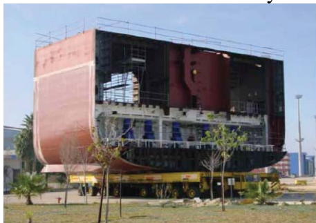
Figure A - Typical block under construction in Spain ~462 tonnes.
