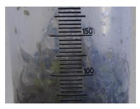
Dry test. The 400+ shrimp were placed into the jug and after the shrimp stopped jumping around the volume was observed to be approximately 100 ml.
