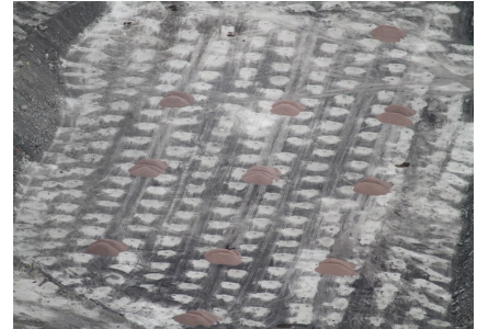
Sonoma Coal Mine on Coral Creek Beside Bowen Developmental Rd. Shot firing/Blasting preparation.
