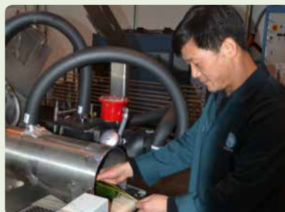
Dr Xinqing Xu feeding the microwave unit with zucchini fruit (with fibre optic cables for online temperature measurement during treatment).
