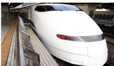
The specialised beak of the Kingfisher, which allows it to move from air to water with minimal noise or splash, provided engineers with a design solution for the 200 mile an hour bullet train, enabling it to be quieter and more energy efficient.
