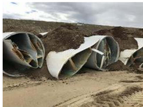
Disposing of cutup wind turbine blades
