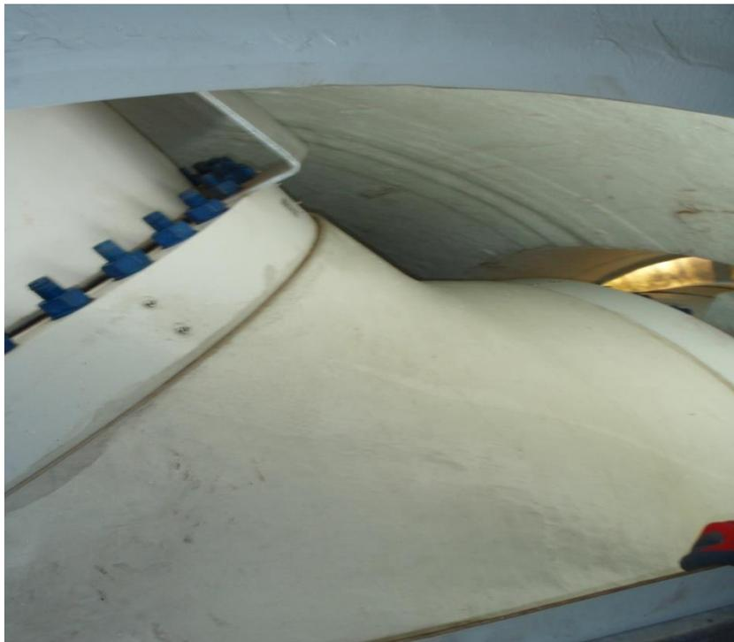
Figure 9- Depicts the Hub and blade connection. Cone over the outside.
