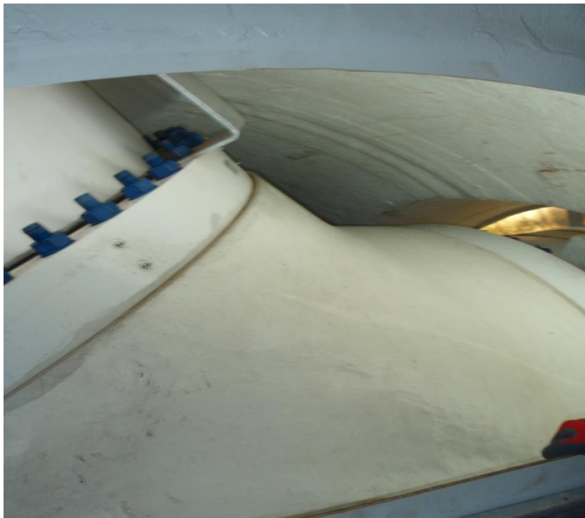
Figure 9- Depicts the Hub and blade connection. Cone over the outside.
