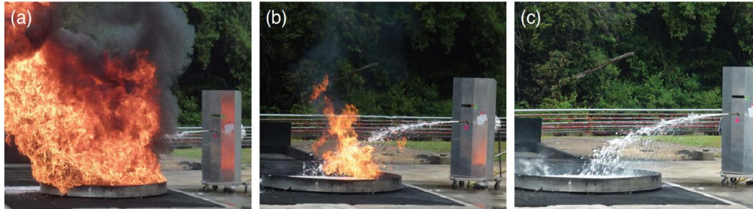
Effective ICAO Level B Fire test demo using C6 AFFF at Singapore Fire Conference, July 2016.
