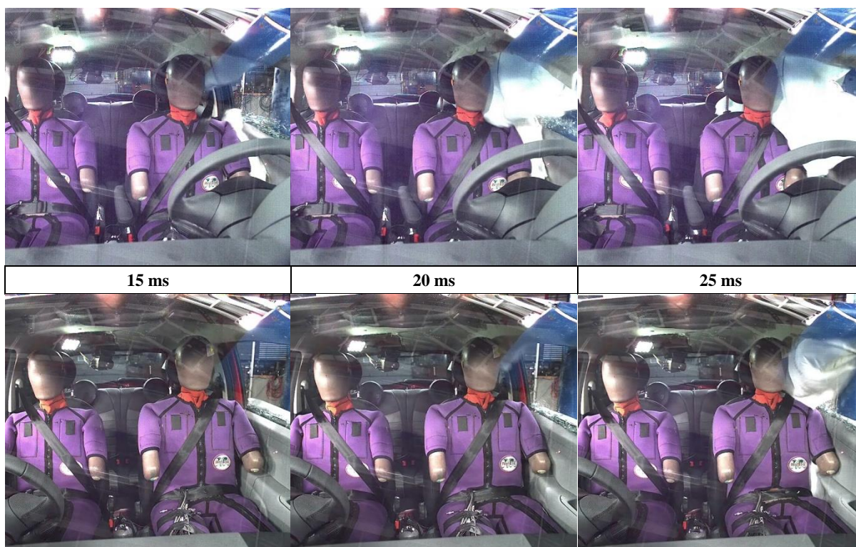
Figure 15 North American market vehicle (top row) and Australian market vehicle (bottom row) side airbag deployment, 15-25 milliseconds after first vehicle contact with the pole, during an oblique vehicle-to-pole side impact test (Model A)
