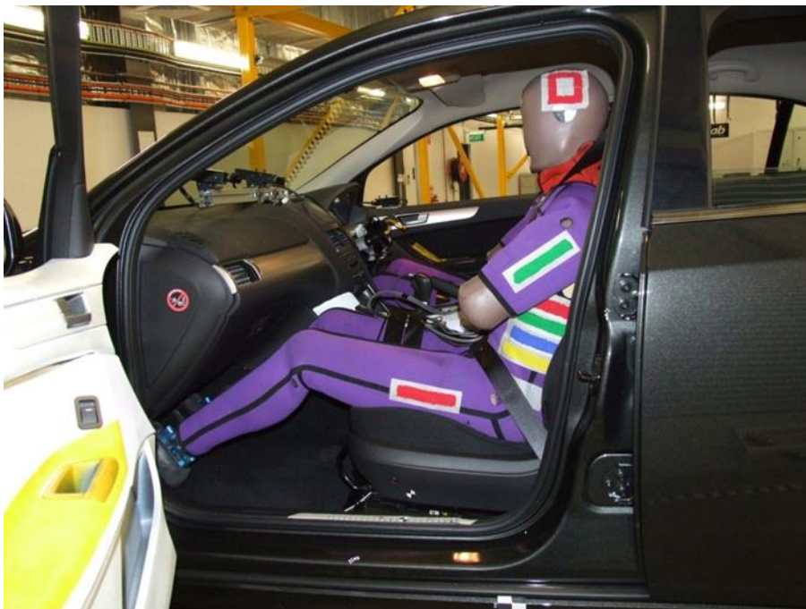
Figure 9 A WorldSID 50 th percentile adult male positioned in a large passenger car
