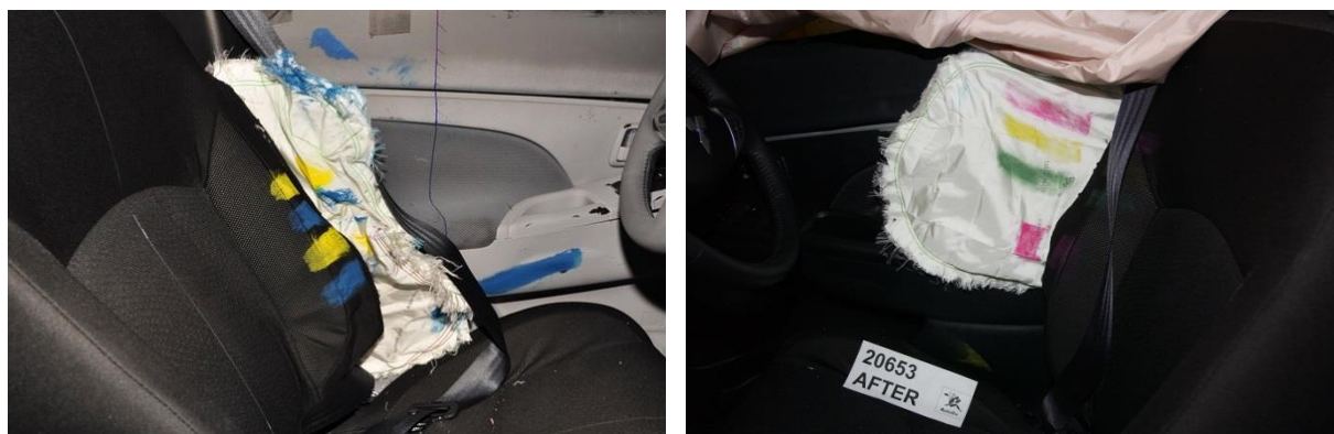
Figure 16 North American market vehicle (left) and Australian market vehicle (right) thorax side airbags, post deployment (Model B)
