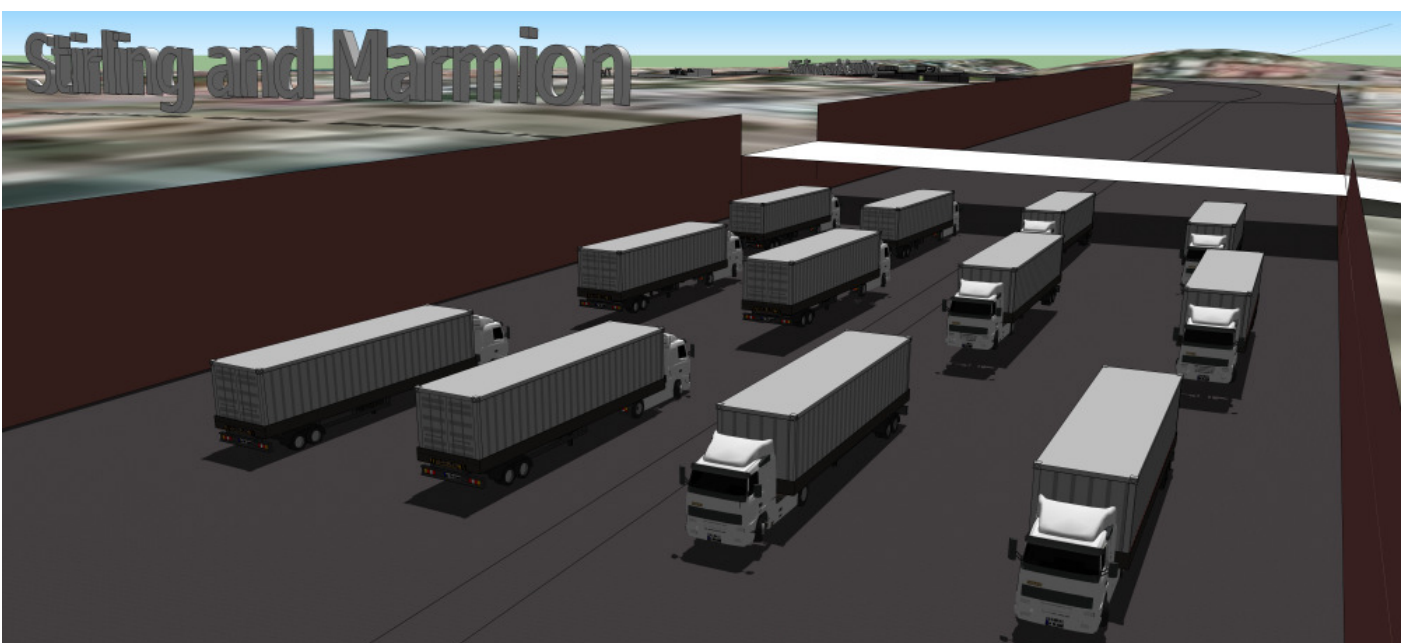
Figure 15. The new proposal for Stirling Highway as it passes under Marmion Street. at this point it is 6.5 meters deep.
