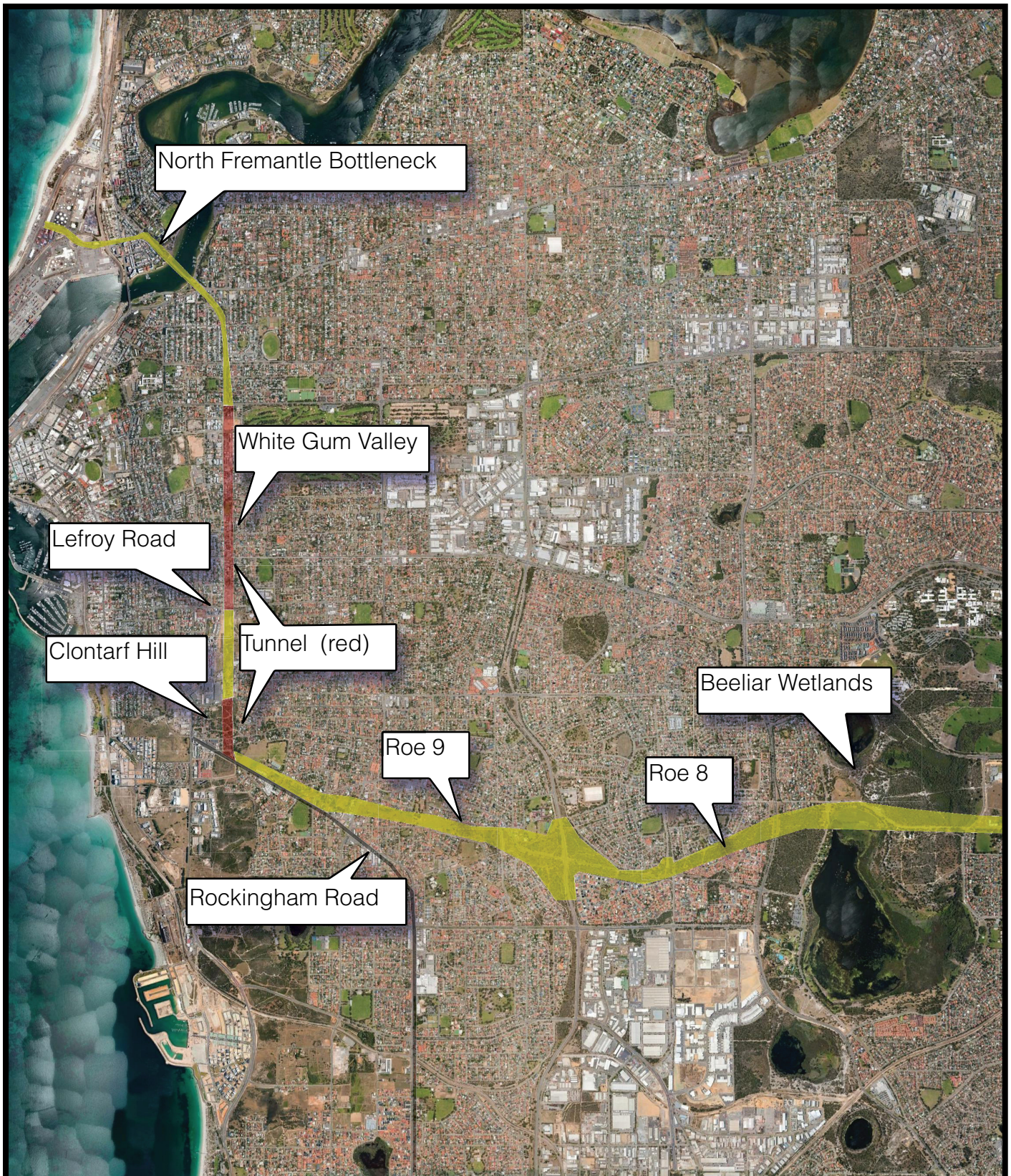
Figure 19. The Road Tunnel option as an extension of the Roe 8 and Roe 9. In red are the likely tunnels, under Clontarf Hill and White Gum Valley and in yellow will be the 'at grade' highways. What is also apparent is the degree to which the width and speed of the Roe Highway will be reduced once it arrives into a tunnel to then enter the Port of Fremantle where truck congestion awaits.
