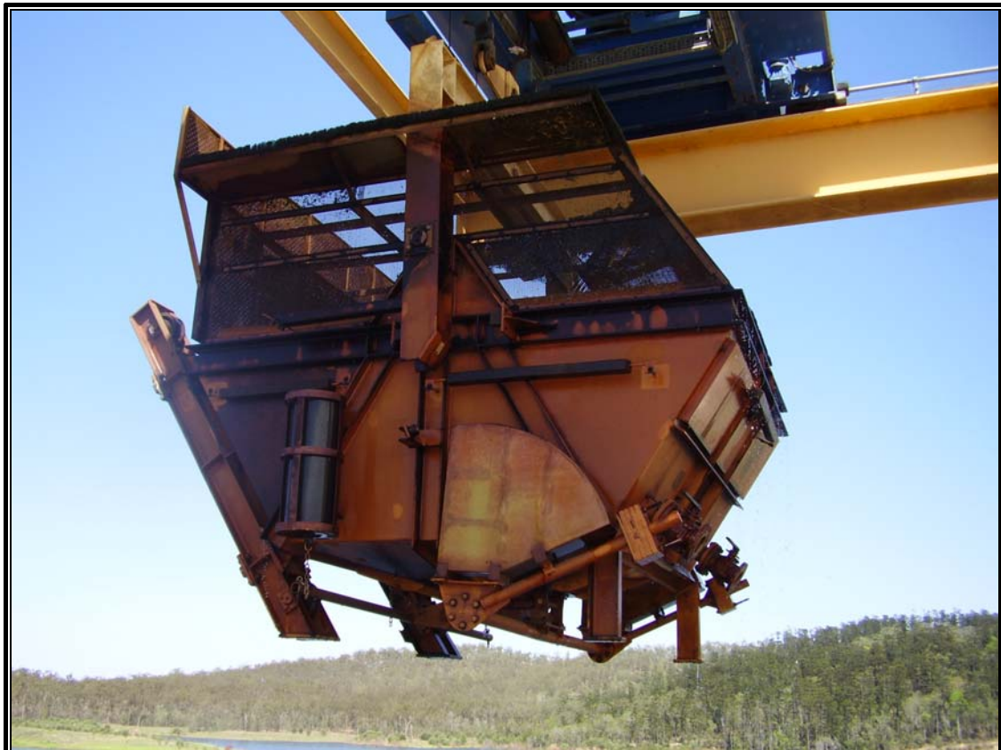
Images of upstream fish passage cage , ready to be lowered behind the dam wall
