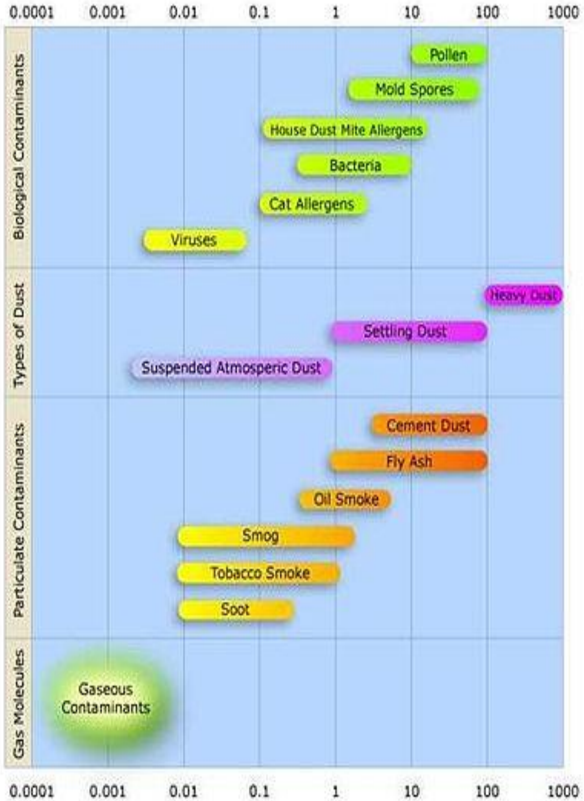
This diagram shows the size distribution in micrometres of various types of atmospheric particulate matter. It also shows the different types of particulates in the atmosphere. Wikipedia 'Particulates'
