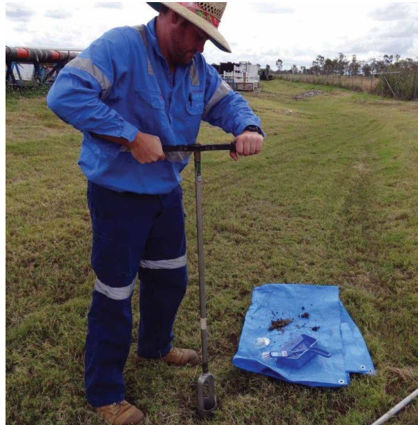
A hand auger is used to drill small bore holes during geotechnical investigations.
