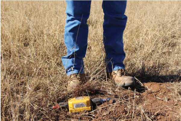
Wireless geophone and battery pack.
