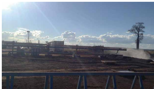
Blooie line during underbalanced drilling.
