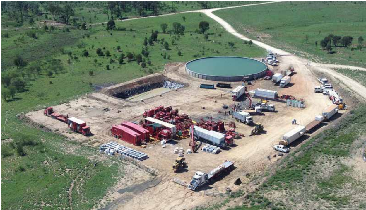
Lease layout during hydraulic fracture activities, commonly known as a ‘frac spread’.
