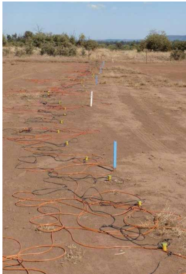
Geophones and lightweight cables along a seismic line.
