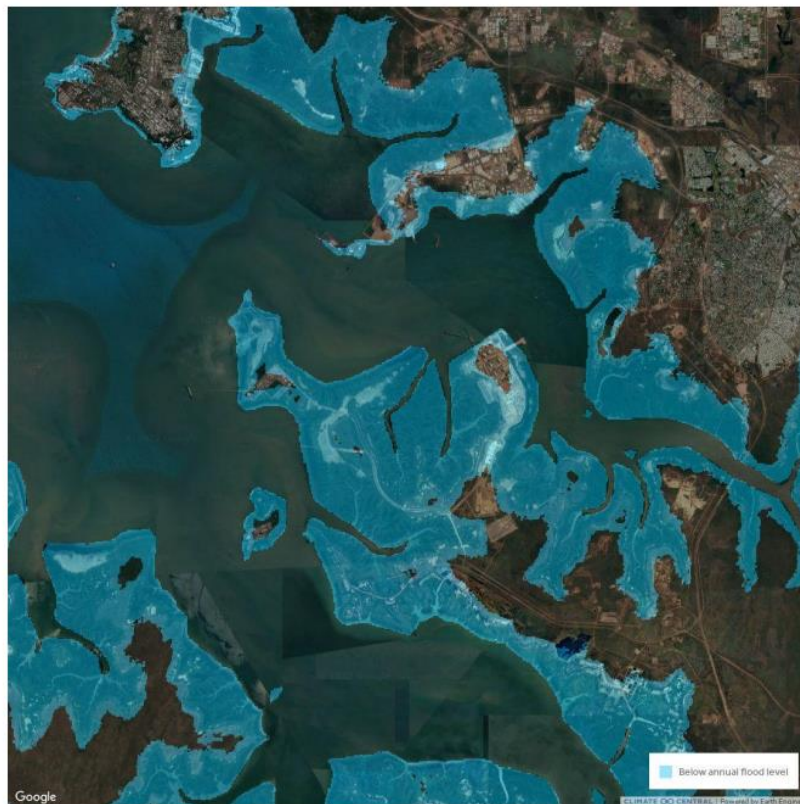
Figure 1. Mid-range sea level rise projection shows that by 2030, annual flooding will reach areas planned for industrial facilities within the Middle Arm Development. 16
