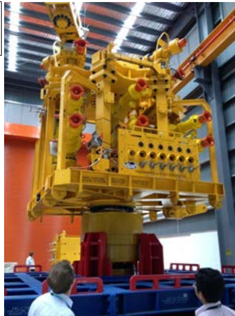
Figure 6: 'Cap and containment' technology Source: OSRL
