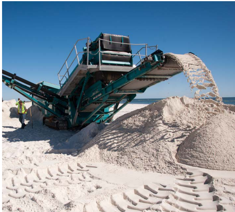
A "PowerScreen" machine cleans an area of Orange Beach, Ala. and returns cleaned sand to the beach in 2010.
