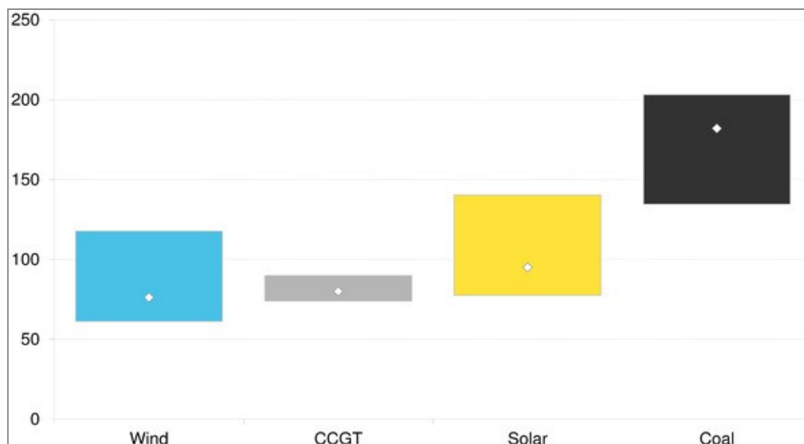
Figure 1: 2017 levelized cost of energy for new build technologies in Australia (AUD/MWh)
