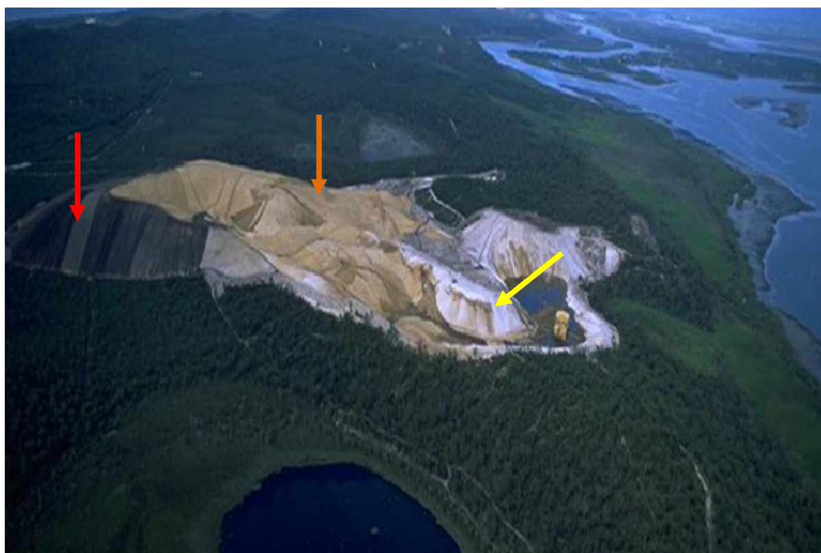
Figure 7: Oblique aerial view to south of Gordon Mine (not in active operation today). Note the exposed soil profile in dredge-pond walls (yellow arrow), brown-coloured tailings of homogenised sand (orange arrow) and grey topsoil spread ready for revegetation (red arrow). (Photo by CRL)
