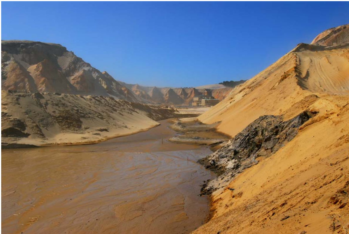
Figure 11: Enterprise Mine working area with floating dredge in distance and partially mined dunes in foreground and mid-ground. Photo by FOSI (2009)
