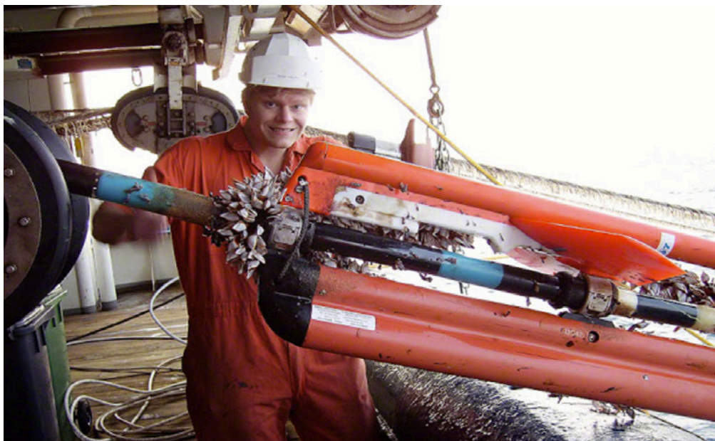
Fig 12. Barnacle growth on streamer depth controller.
