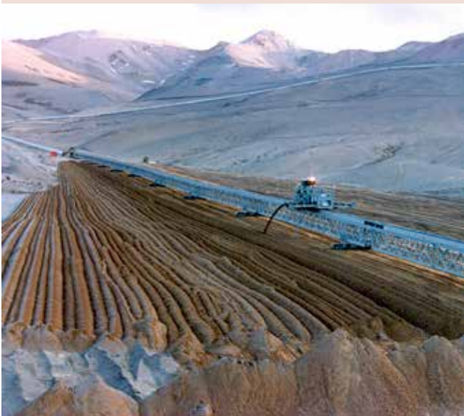
Dry stacking at the currently closed La Coipa gold and silver mine in Chile (installed 1990) with a capacity of 28 800 tonnes per day
