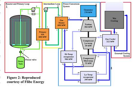
deactivate itself. The freeze valve located in Area 1 (fig.2) makes the system passive, if the reactor stopped the valve would melt and the drain tank would fill(WNA,2018).
