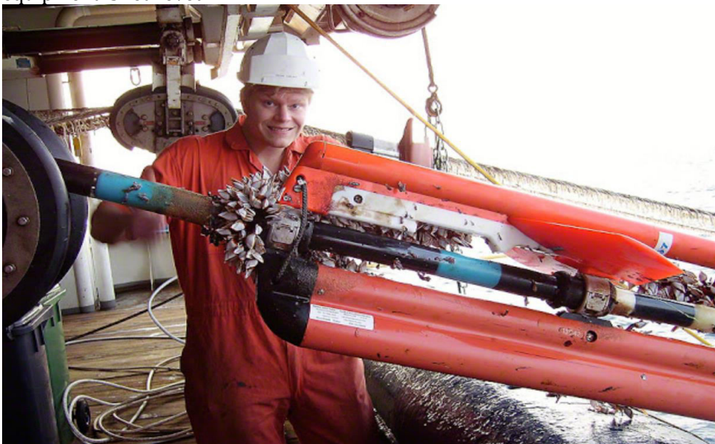
Fig 12. Barnacle growth on streamer depth controller.
