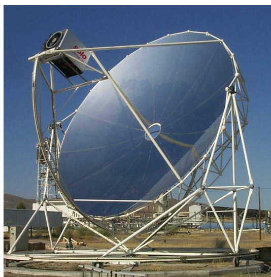
Figure 3.13: Picture of a solar parabolic dish to provide heat to a Stirling generator (Wikimedia, 2009c)
