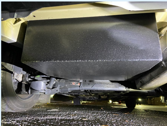
Victoria – Peugeot Partner – Hydraulic hide under rear storage area.
