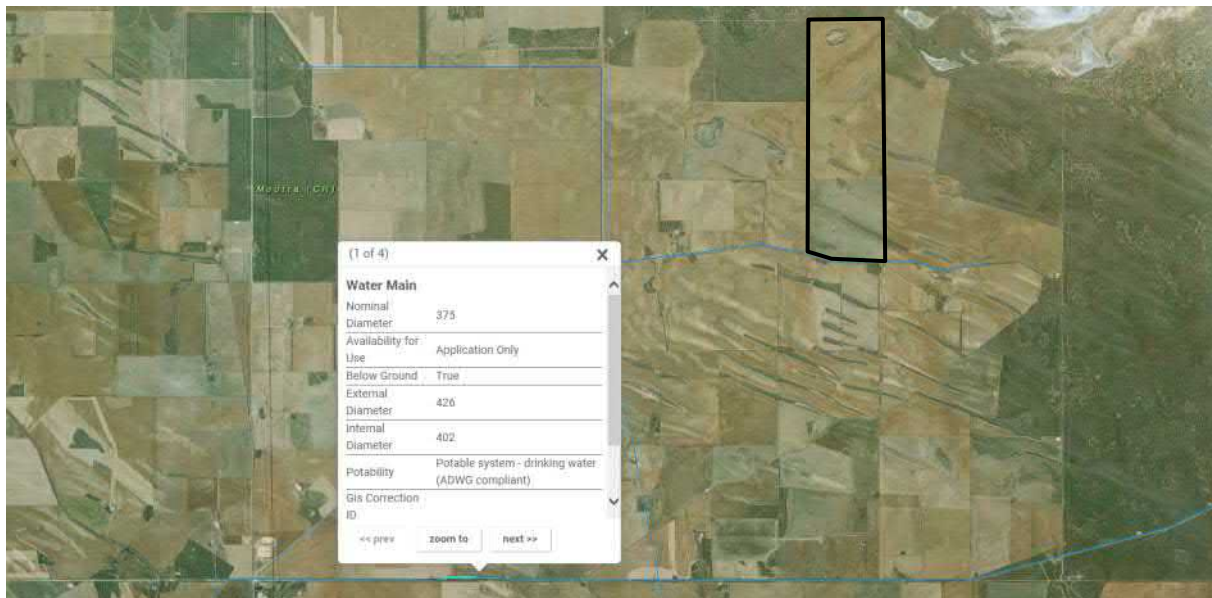
Figure 51 Location SA MapViewer screenshot showing the site location in relation to the nearest water main
