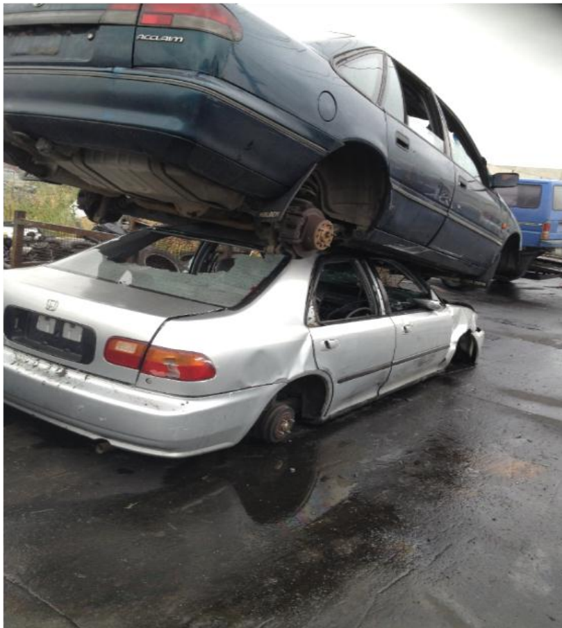
21.3 Figure 23: Substantially non-compliant worksite, vehicle bodies stacked unsafely
