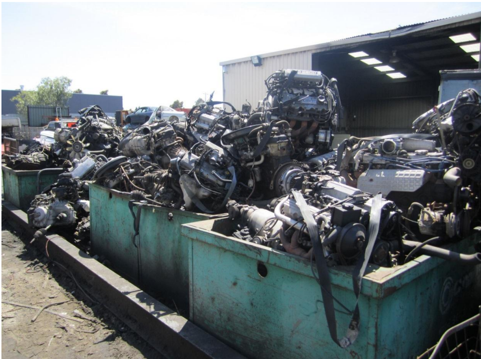
20.3 Figure 19: Mostly compliant worksite, storage bins are in a bunded area but bins are too full and parts are stacked too high
