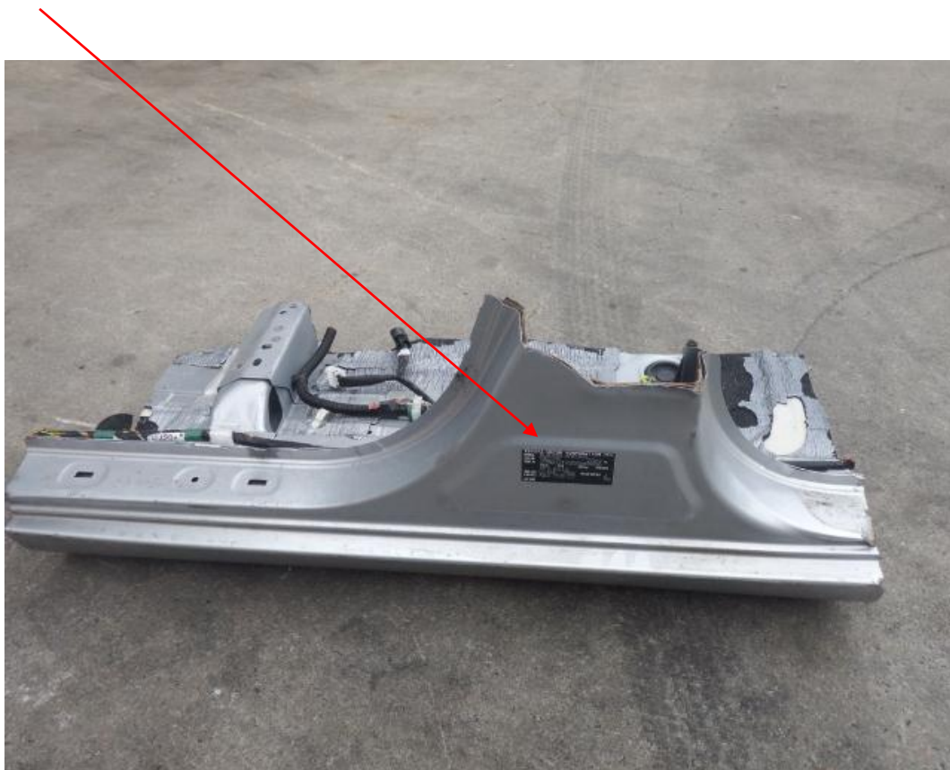
14.4 Figure 11: Section of sill and 'B' pillar from a stolen Toyota RAV4, build plate attached
