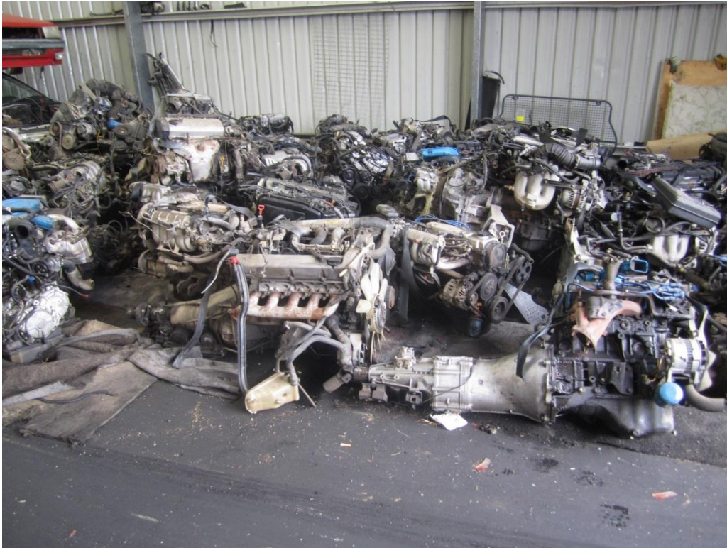
22.3 Figure 27: Completely non-compliant worksite engines stored on worksite floor, lack of bins or storage containers
