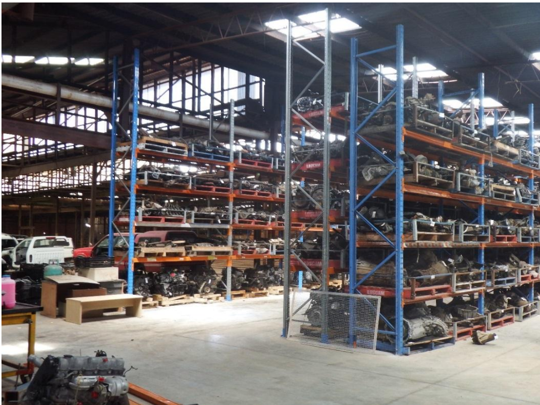
19.4 Figure 16: Substantially compliant worksite with stable storage and shelving
