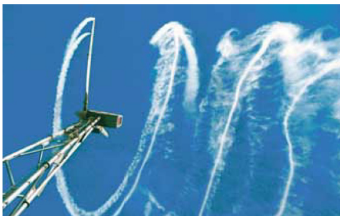
Wake effect. Source: Danish Wind Energy Association Guide, 2003, pg. 34
