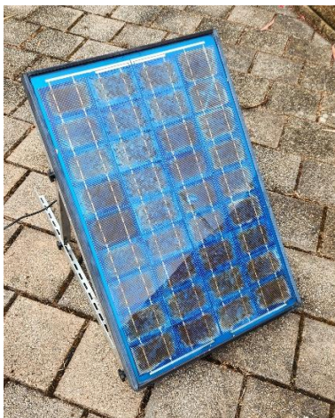
Figure 1: 33 Year old Australian Made Solarex 40W Panel
