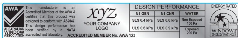
Figure 2.7 105 x 16 mm Type 2 Performance Label on Silver Matte Mylar.
