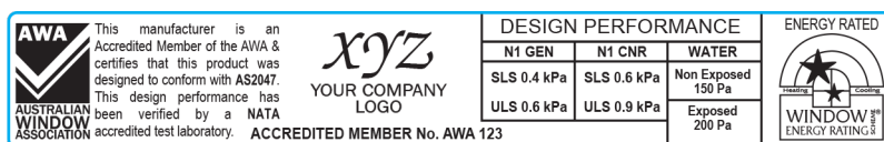
Figure 2.6 105 x 16 mm Type 2 Performance Label on Clear Mylar.
