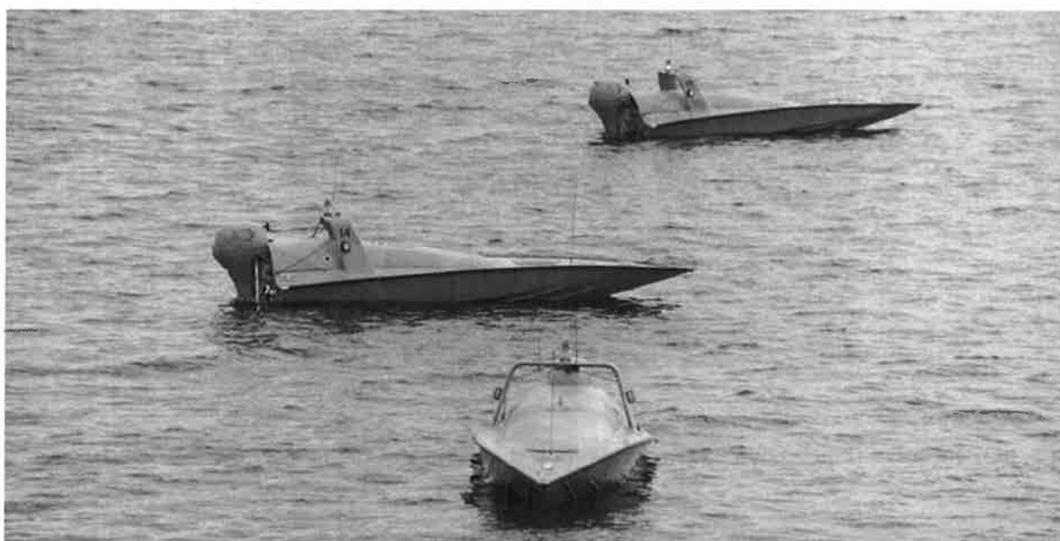
Figure 3: Saab Kockums' Piraya (swarm) Unmanned Surface Vessels
