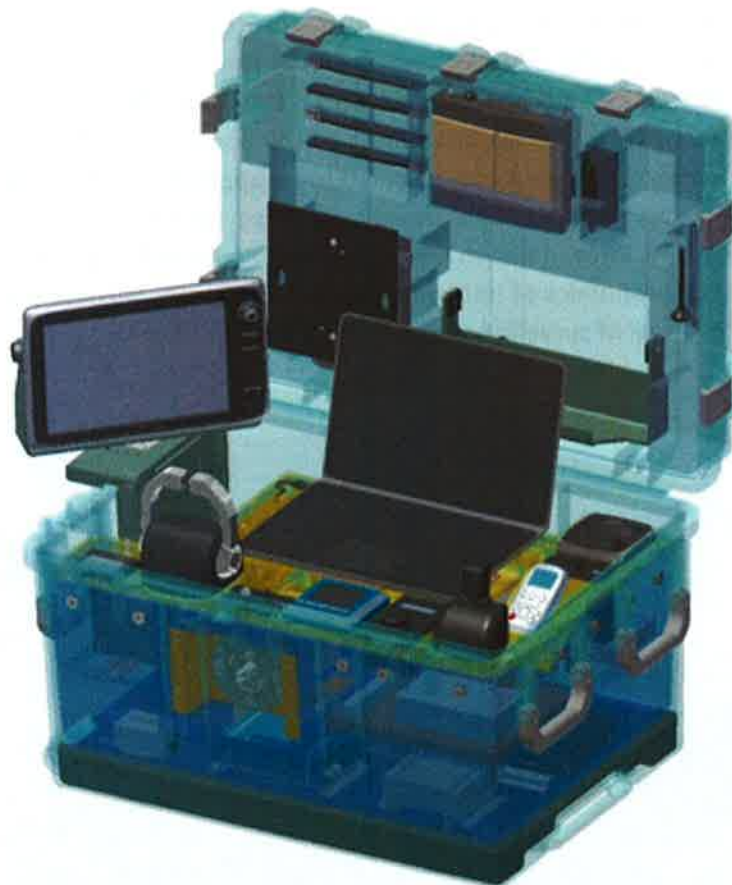
Figure 3: Illustration of the deployable Control Station that is part of the flexible Mission Management System for USV control
