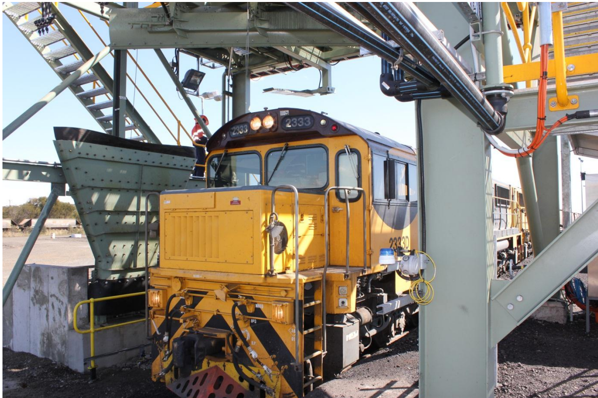
Close up photograph as a train enters the profiling and veneering station.
