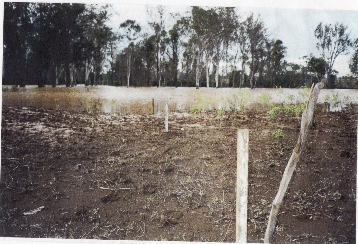
Bracewell Lake - distance between stakes Represents daily absorption rate
