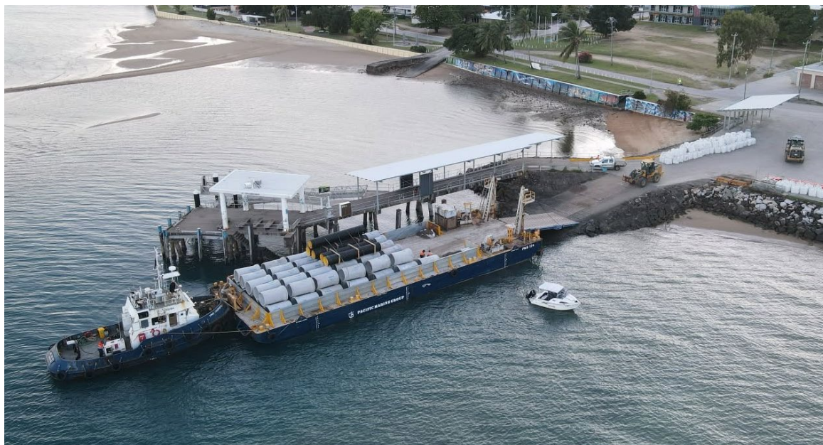
(1) Tug and Barge operation - Palm Island Barge Ramp. Note tug is used to push barge onto the concrete barge ramp, then the bow door is lowered. A set of fender piles along the port (left) side of barge align the barge onto the ramp
