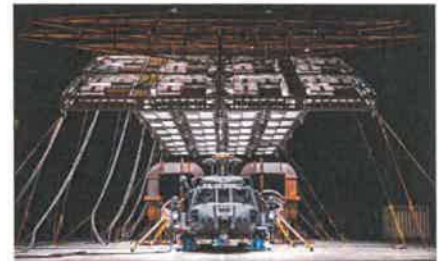
An HH-60W Jolly Green II sits under bright lights used to create heat in the McKinley Climatic Lab at Eglin Air Force Base (AFB), Florida (March 19, 2020).
