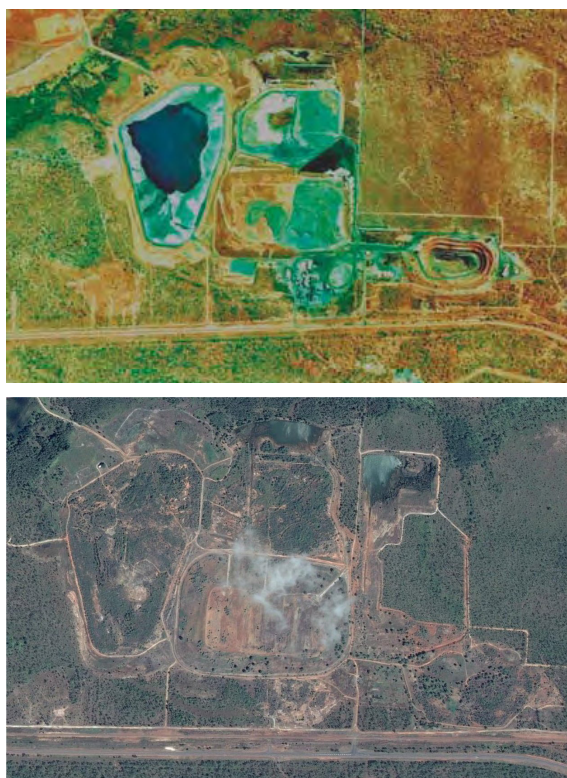
Figure 9: Aerial views of the former Woodcutters Pb–Zn–Ag mine, NT—(top) prior to rehabilitation in 1998 (Taylor & Pape, 2007); (bottom) recent site view 17 May 2016 (GE, 2016) (note: north is pointing to the right)
