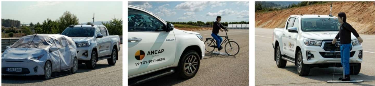
Figure 8 - AEB Scenarios: Car-to-Car rear, Car-to-Cyclist and Car-to-Pedestrian
