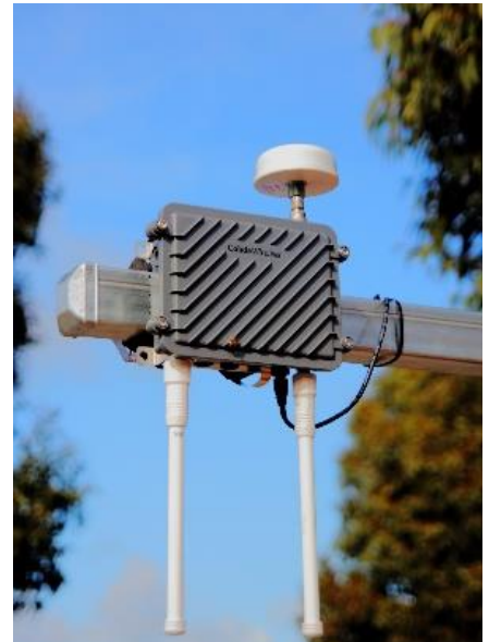
Figure A2: Roadside infrastructure for vehicle-to-infrastructure communications
