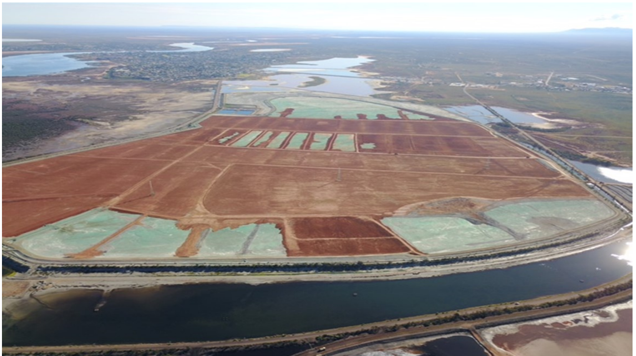
Figure 4 Ash Storage Area as at June 2017 demonstrating the access finger construction and spreading approach
