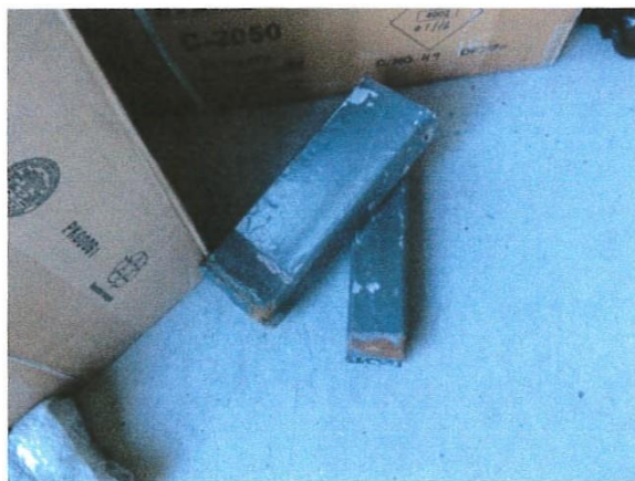
Asbestos products found at the Executive Building Site, Brisbane
