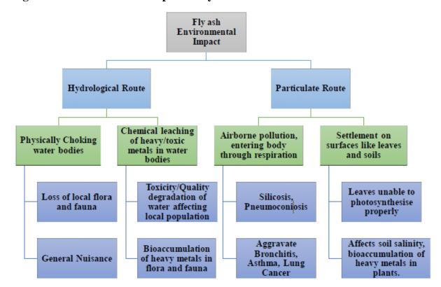
Figure 9.1 Environmental impact of fly ash<sup>14</sup>
