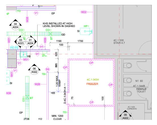
(b) For the existing Services use MicroStation: 112 (RGB 150,150,150), AutoCAD: Colour 253 (RGB 153,153,153). The example below shows new services in colour and the existing architectural elements and services in greyscale.
