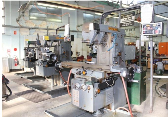
**Vertical turret milling machine (Hunter TAFE has 12 vertical turret milling machines)**
