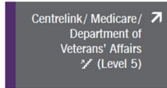
SIGN 2 QTY: 1 Computer cut vinyl graphics applied to 4mm clear acrylic 800mm X 400mm
