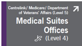
SIGN 2 QTY: 1 Computer cut vinyl graphics applied to 4mm clear acrylic 770mm X 415mm
