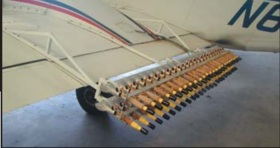
Wing-mounted pyrotechnic flares are used to distribute seeding materials into clouds in Texas. Photo: John Forrest
