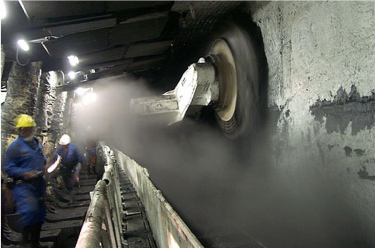
An example of dust control in a longwall mine.<sup>21</sup>
