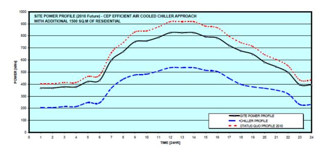
Graph 1: The estimated site power profile for 2010 with the Central Energy Plant and low load Thermal Energy Storage, showing a reduced power profile (black line) as opposed to the business-as-usual profile (red dotted line).
